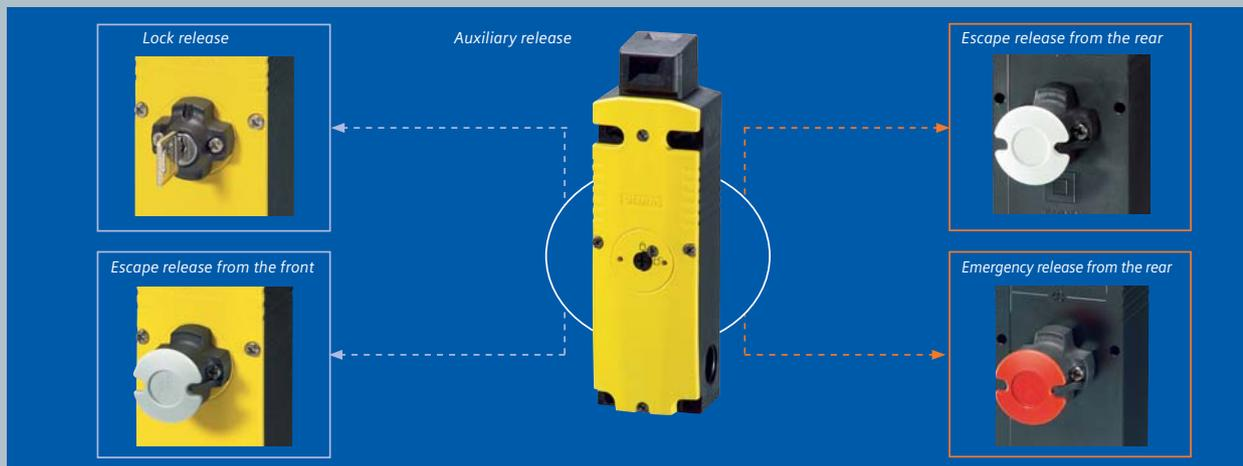
The escape release facilitates a manual unlocking of the interlocking to enable persons to leave the hazardous area – without auxiliary equipment from the escape side, i.e. inside the hazardous area. The emergency release facilitates the manual unlocking of the interlocking in cases of danger – without auxiliary equipment from the access side, i.e. outside the hazardous area.
